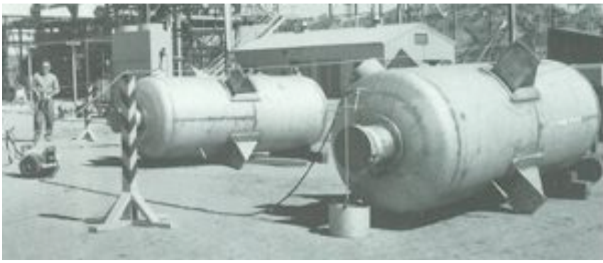
Here, a portable iridium-192 source is being used for gamma graphing of weldments on field installations. It also has a 3½-curie cesium gamma graphing apparatus, and also has a 5-curie cobalt-60 source, for the examination of dense materials.
