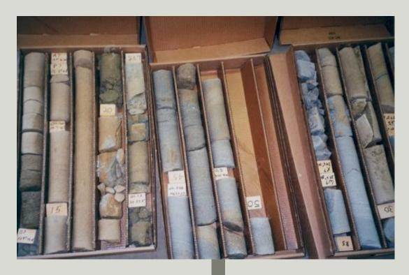
100s of samples are collected from each core and analyzed for volatile organic compounds providing detailed profiles of the chemicals in the rock.
