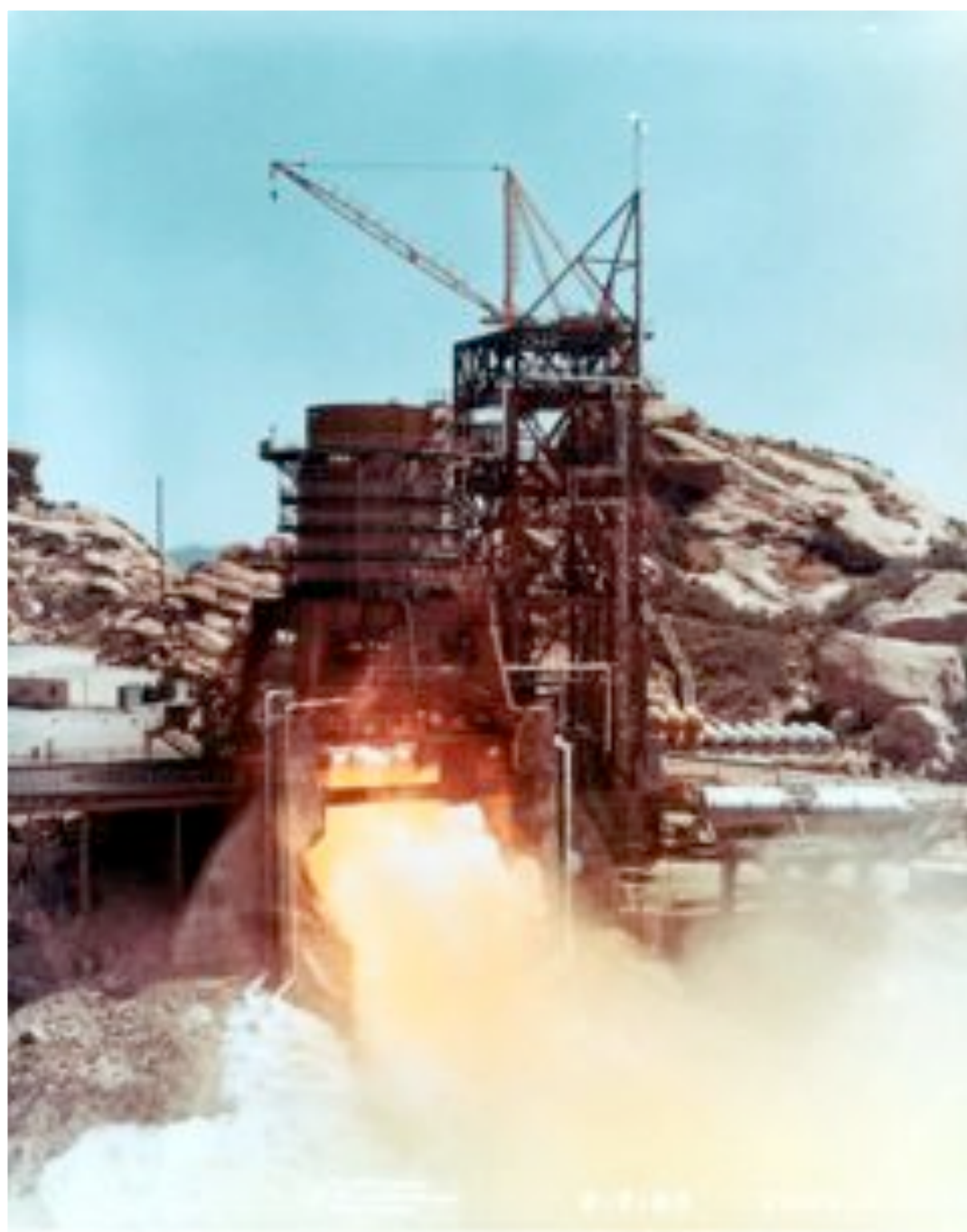
Coca Test Area - S-II Battleship J-2 Five Engine Cluster Hot Fire Test - 1955
