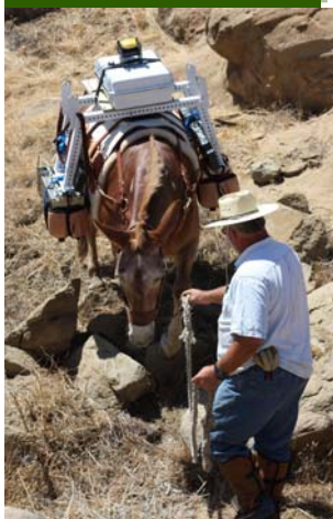
EPA's mule-mounted gamma scanning technology at work in Area IV at SSFL.
