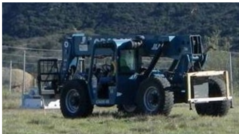
Enhanced Radiation Ground Scanner (ERGS) II gamma scanning technology at work in Area IV at SSFL.
