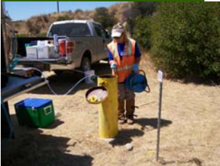
EPA contractor gauging a well during the August groundwater sampling event.
