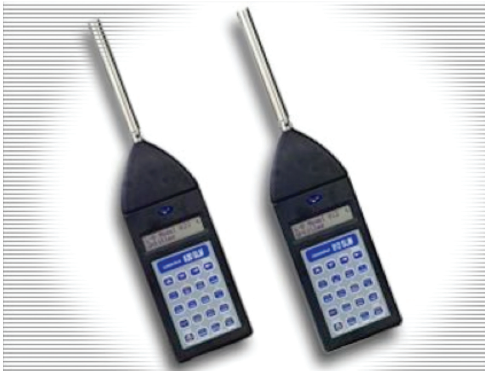
Noise monitoring activities will use noise monitors like these to measure sound levels associated with passing vehicles.
